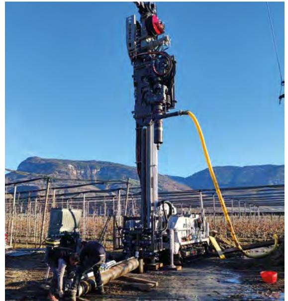
Eurodrill is not only interested in replacing the usual diesel engines with electric motors, but also in the electrification of the largest consumer of energy within the rig – the drilling head.
